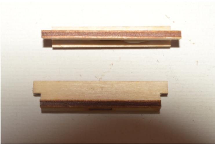
Glue the 2 parts that make up the end frame spacers as shown.
